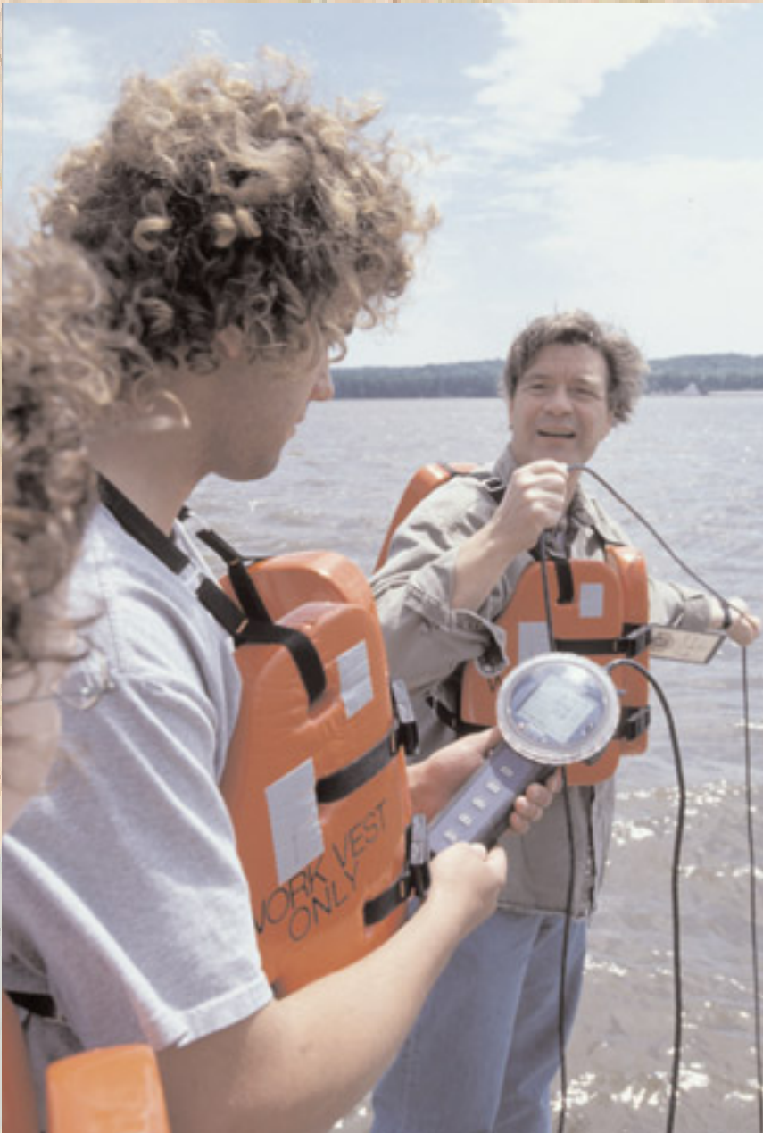
Top: On the banks of the Mississippi River, Professor Jerry Schnoor shows students how to use a Hydrolab, a probe that measures a number of characteristics that help indicate water quality. These include pH balance, conductivity, depth, and temperature.
