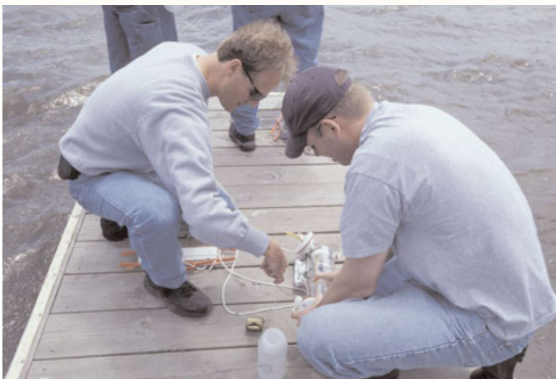
Craig Just (left), senior research assistant in civil and environmental engineering, helps a student prepare the Van Dorn water sampler. Students lowered the apparatus into the Mississippi River near the Lucille A. Carver Mississippi Riverside Environmental Research Station to secure water samples for a chemistry lab.
