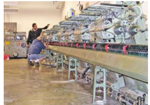
Printing employees Jerry Kilts, background, and Mike Woodhouse adjust the saddle stitcher after moving it to the bindery's new location.
